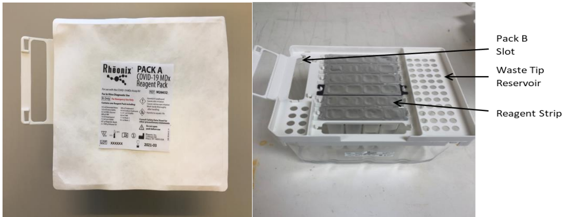
Figure 3. Rheonix COVID-19 MDx Assay Pack A. Left: Pack A after being removed from assay kit box and with its Tyvek lid in place. Right: Pack A with the lid removed and various aspects of the pack called out on the right.
